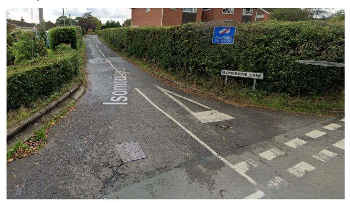
**Detail:** Remove central lining and replace with cobble strip to visually change width of road and slow drivers down when accessing and exiting Isombridge Lane. Location: ///proofread.pasting.outboard
