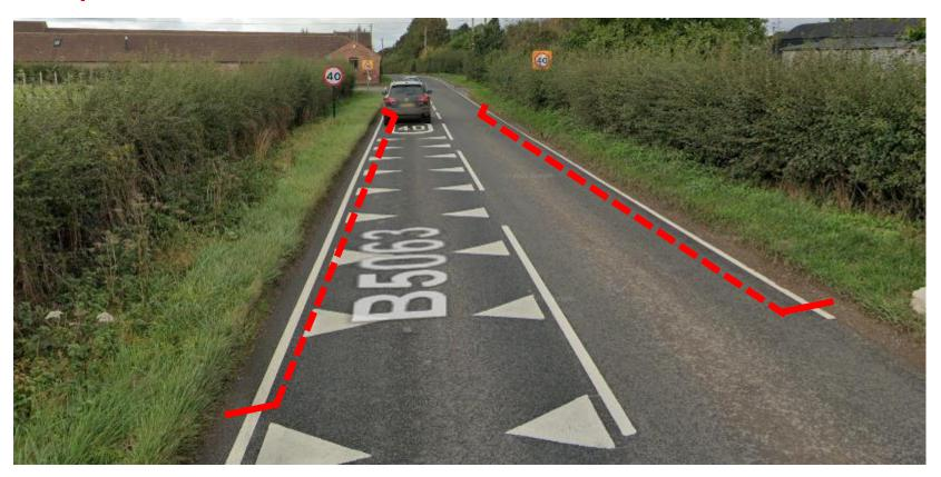
**Detail:** Change 40mph to 30mph before entering main built up areas of Longdon upon Tern. Clear current markings and replace with hatching each side to visually narrow road. Location: ///jiffy.wiggly.linguists
